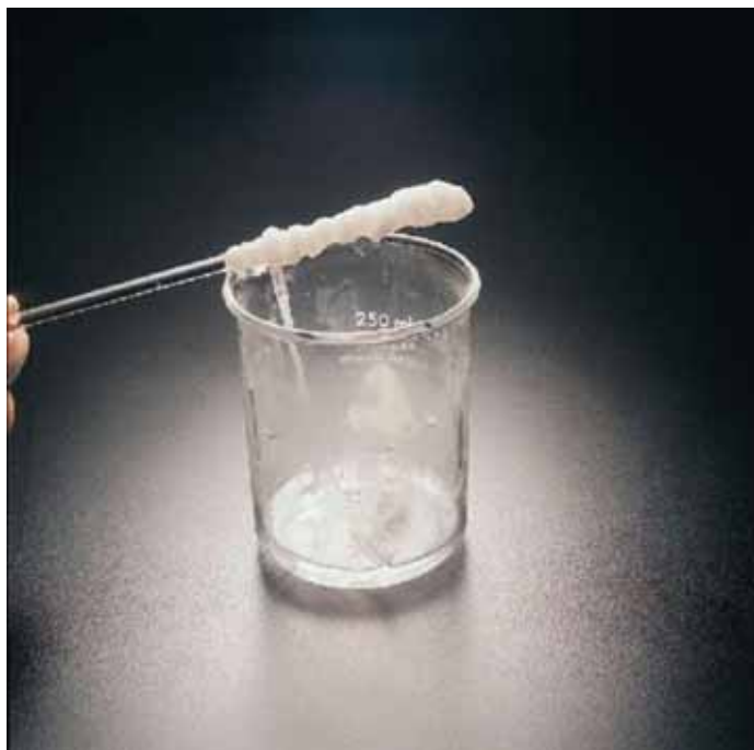
Figure 2.17 Nylon-6,6. Hexamethylenediamine is dissolved in water (bottom layer), and adipoyl chloride (a derivative of adipic acid) is dissolved in hexane (top layer). The two compounds react at the interface between the layers to form nylon, which is being wound onto a stirring rod.
