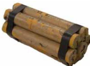
Figure 2.6 Nitroglycerin. (a) Concentrated nitric acid and glycerin react to form an oily, highly unstable compound called nitroglycerin, \text{C}_3\text{H}_5(\text{ONO}_2)_3 . (b) Nitroglycerin is more stable if absorbed onto an inert solid, a combination called dynamite. (c) The fortune of Alfred Nobel (1833-1896), built on the manufacture of dynamite, now funds the Nobel Prizes.
