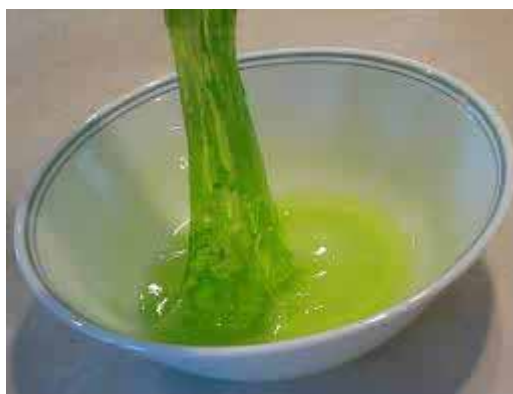
Figure 2.14 Slime. When boric acid, B(OH)_3 , is added to an aqueous suspension of polyvinyl alcohol, (CH_2CHOH) , the mixture becomes very viscous. This is because boric acid reacts with the -OH groups on the polymer chain, causing cross-linking to occur. (The model shows an idealized structure of a portion of the polymer.)
