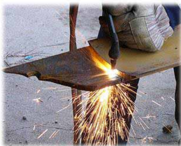
Figure 2.4 An oxy-acetylene torch. The reaction of ethyne (acetylene) with oxygen produces a very high temperature. Oxy-acetylene torches, used in welding, take advantage of this fact.
