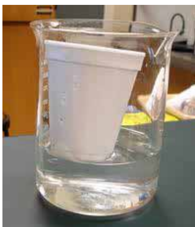
Figure 2.13 Polystyrene (a) The polymer is a clear, hard, colorless solid, but it may be more familiar as a light, foamlike material called Styrofoam. (b) Styrofoam has no polar groups and thus dissolves well in organic solvents such as acetone.
