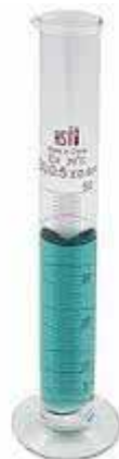
Figure 3.4 The level of a liquid in a graduated cylinder. The saucer-shaped surface of a liquid in a tube is called a meniscus.
